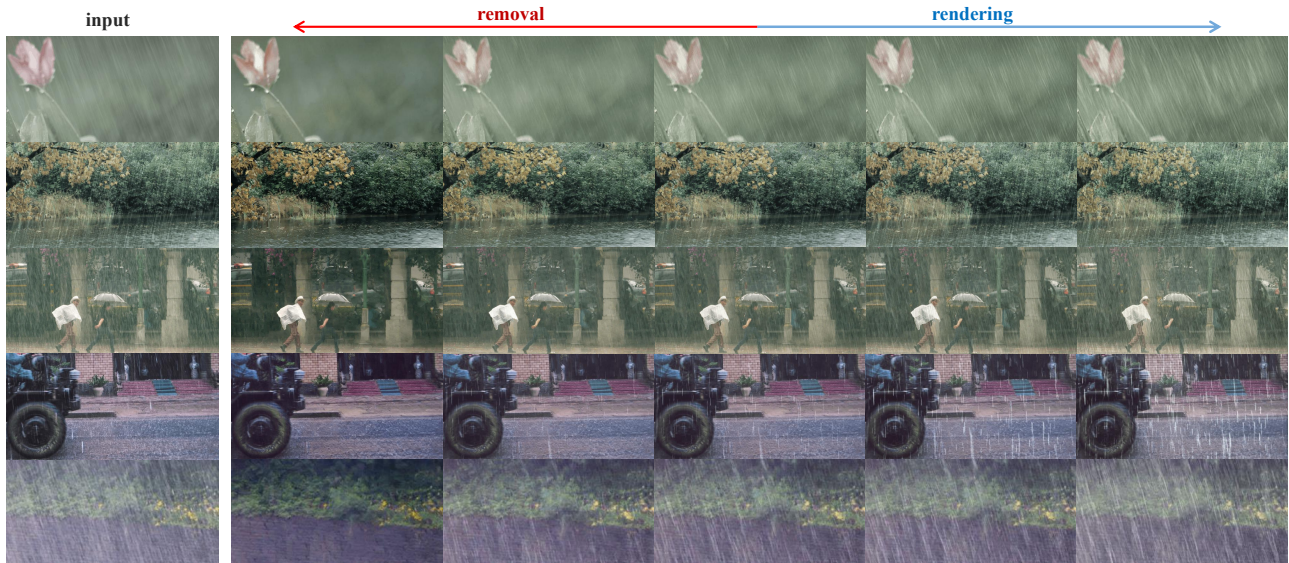
Figure 8. Bi-directional and continuous rain control results on real rain images.
